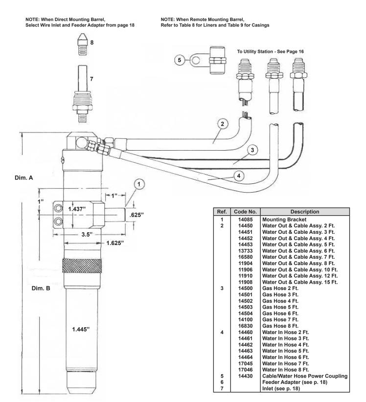
NOTE: Water-Cooled Nozzle selected determines length in 1" increments.
